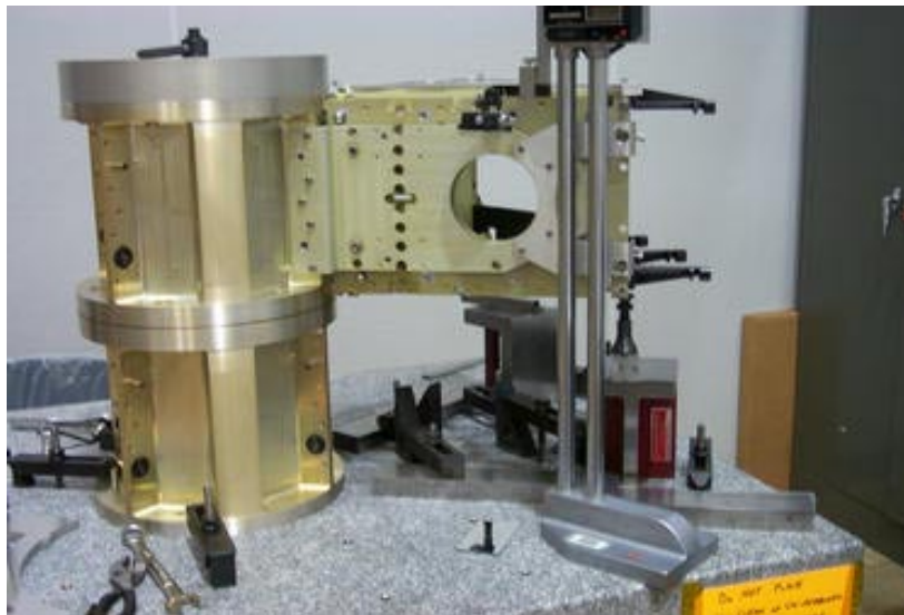
Fig. 12: OAP Primary Optic Housing assembly process.
