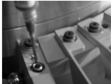
Fig. 14: Example of mounting bushing assembly technique.
