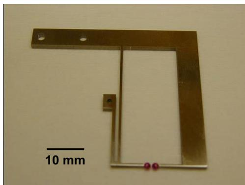
**Figure 2.** One of three double-sided flexures for the thin foil holder.
