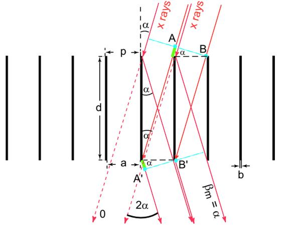
Figure 1. Schematic cross section through a CAT grating. The  $m^{\text{th}}$  diffraction order occurs at an angle  $\beta_m$  where the path length difference between  $AA'$  and  $BB'$  is  $m\lambda$ . Shown is the case where  $\beta_m$  coincides with the direction of specular reflection from the grating bar side walls ( $\beta_m = \alpha$ ), i.e., blazing in the  $m^{\text{th}}$  order.
