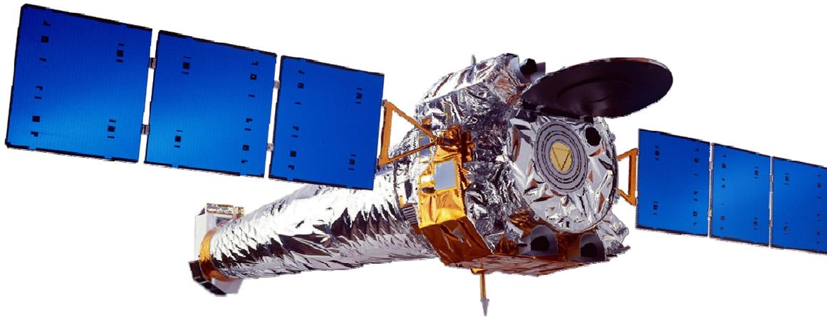
Figure 1. NASA's *Chandra X-ray Observatory*: 13.8-m length, 4.2-m diameter, 19.5-m wingspan, and 4800-kg mass. The *Chandra* flight system comprises the Telescope System (including mirror assembly and optical bench—"tube"), the Spacecraft Module (surrounding the mirror assembly at one end of the optical bench), and the Integrated Science Instruments Module (containing two focal-plane detector arrays at the opposite end of the optical bench). [Credits: NGST]
