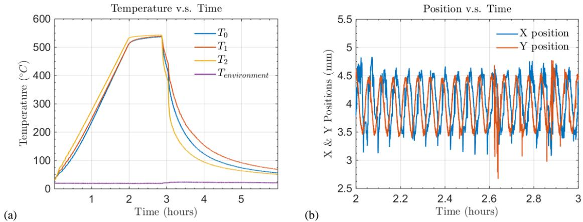
**Figure 6.** (a) Furnace temperature during a slumping run measured at several points near the mandrel. This particular cycle had a peak temperature of around 550 C and peak dwell time of ~0.9 hours. (b) Plot of measured mirror position in the bearing during peak temperature dwell. The control system actuates the hot substrate to follow a ~1 mm diameter “dither” circle with a period of ~3 minutes.
