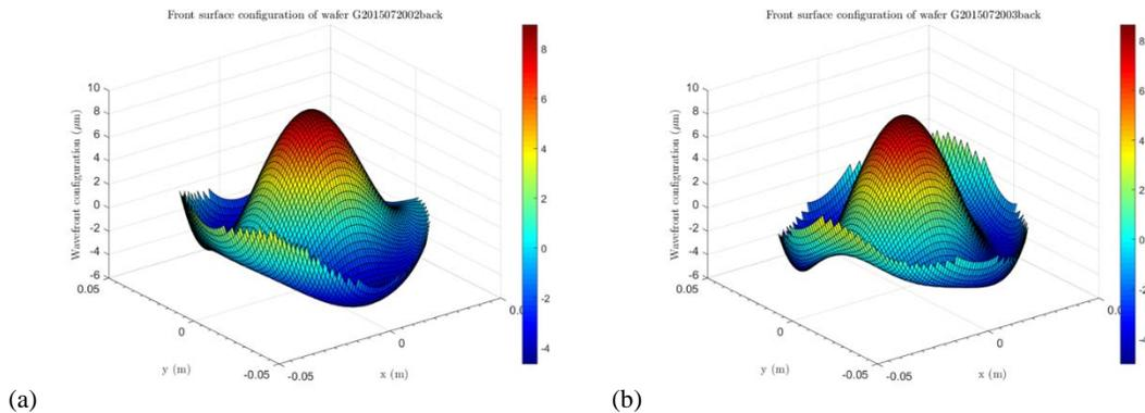
**Figure 8.** Topographs for substrates slumped for 16 hours using a 35 micron bearing gap and a dwell temperature set point of 550 C. (a) Sample G2015072002. (b) Sample G2015072003. Note progression of both samples to a very similar “sombbrero” shape and P-V.
