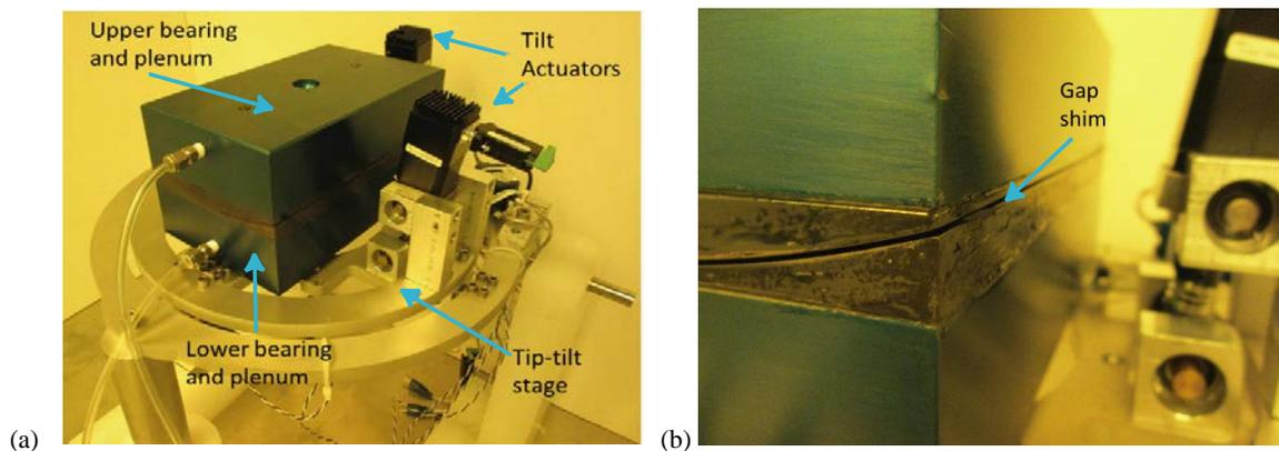
**Figure 9.** (a) Photograph of conical optic slumping test stand which is designed for room temperature tests. This prototype tool is designed to test substrate position sensor and control concepts in a cylindrical geometry. (b) Detail of test stand showing porous graphite air bearings, aluminum plenums and gap shims.
