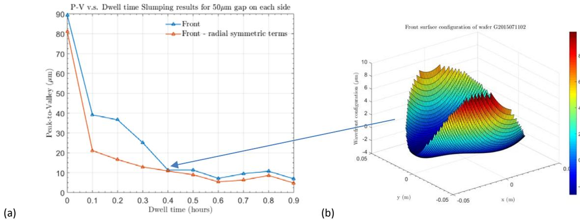
**Figure 7.** (a) Slumping results using a 50 micron bearing gap and a dwell point set temperature of 550 C. Each dwell time trial was performed with a different substrate. Rapid flattening occurs for dwells up to ~0.4 hour duration, which then slows for longer dwells. (b) Shack-Hartmann surface topograph of substrate after an 0.4 hour slump dwell.
