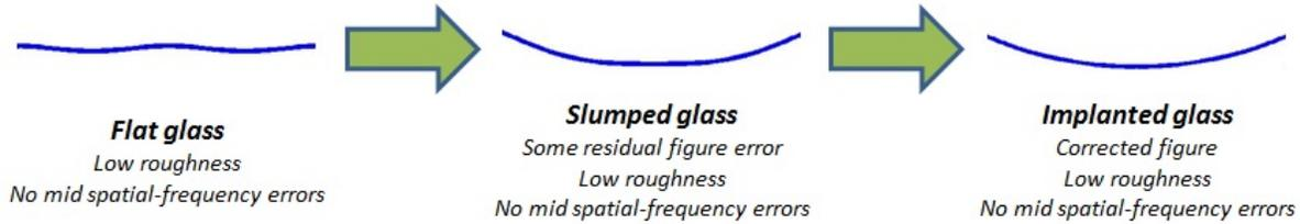
**Figure 2.** Proposed mirror fabrication process. Flat glass is slumped to achieve a figure close to the desired shape, but with very low mid-range spatial frequency errors. A deterministic post-figure correction technique such as ion implant or differential deposition is used to correct remaining figure errors.
