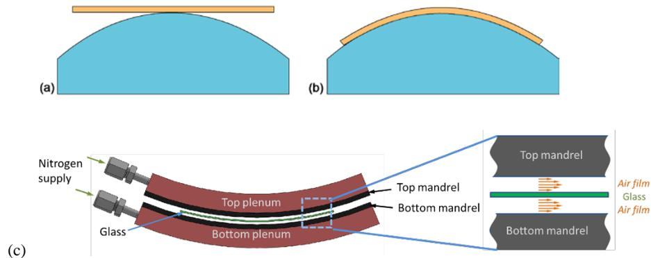
**Figure 1.** (a) Depiction of GSFC thermal slumping process used to produce NuSTAR mirrors. A flat glass sheet (a) is thermally softened and slumped over a precision mandrel (b). (c) Thermal slumping process developed at MIT. Glass is slumped against thin cushions of air generated by a pair of pressurized porous mandrels.
