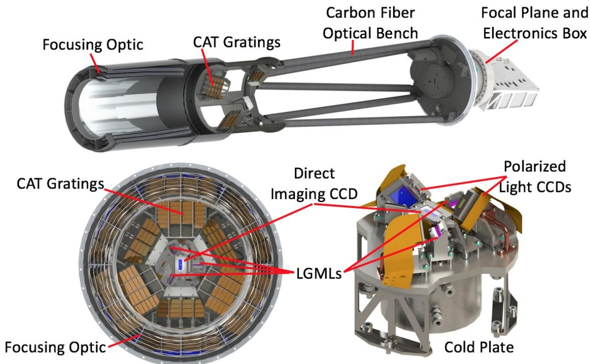
Figure 1. Top: A cutaway of the science payload, showing the locations of the focusing optic, CAT gratings, carbon fiber optical bench and focal plane. Bottom left: a view of the inside of the payload from the aft end looking towards the focal plane. Bottom right: CAD representation of the focal plane, including the liquid nitrogen box on which it sits. Important components are labeled in each image.
