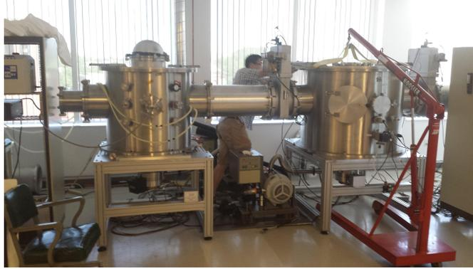
Figure 7. The grating (right) and detector (left) chambers in the new system configuration. The distance between them was originally roughly 10 meters. It is now about 2 meters.
