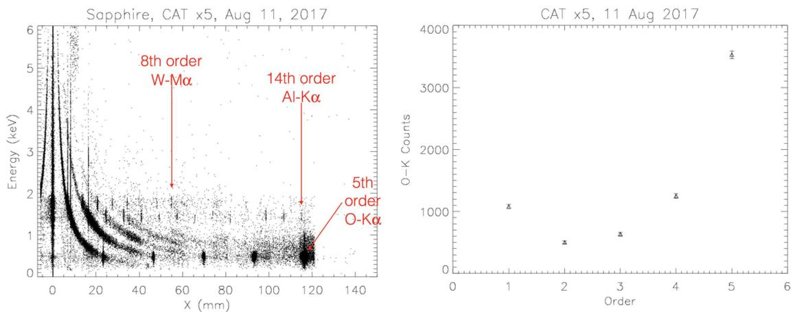
Figure 8. Left: Energy versus position of events on the CCD viewing a Sapphire anode through a slit and CAT grating with the new system configuration. Several orders of dispersion are visible. Right: Counts in the Oxygen K line for several orders dispersed by the CAT gratings. The fifth order contains significantly more power than the lower orders.
