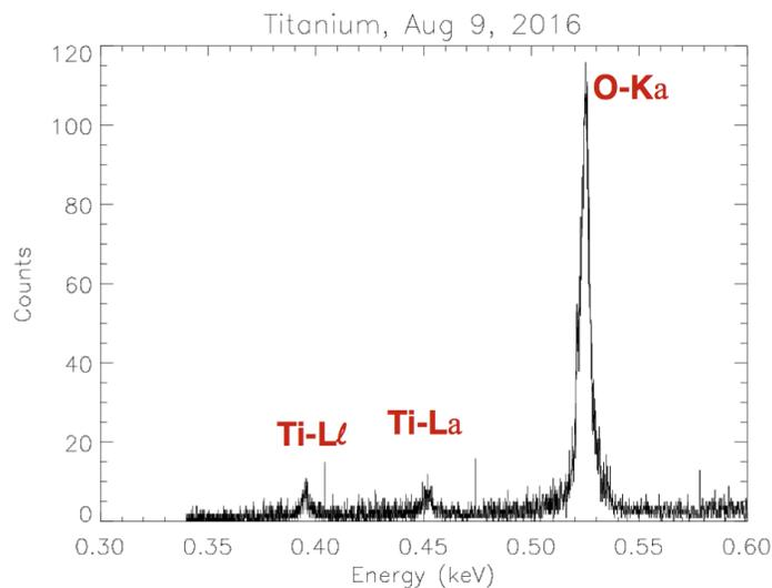
Figure 5. Low energy spectrum acquired using a TiO anode dispersed by a CAT grating. The Ti-L lines are well resolved.
