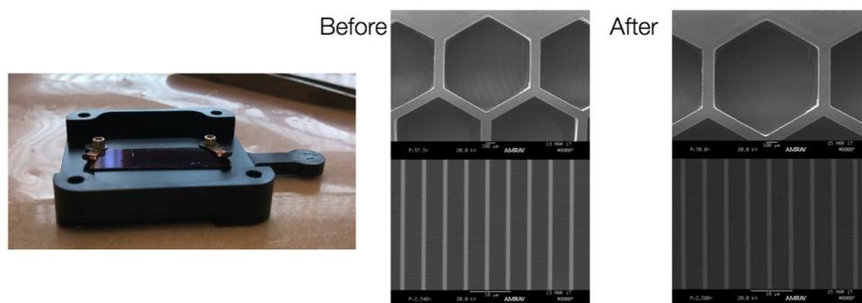
Figure 6. Left: CAT grating mounted on a curved mount, bent with a ROC of 1.5 meters. The mount is designed to mount a curved grating in the system, so that efficiency and spectral resolution can be acquired in the configuration in which the gratings will be flown. Center and Right: before and after SEM images of the grating support structures and bars. The bend does not cause any visible damage to either L1 or L2 support structures or the grating bars.
