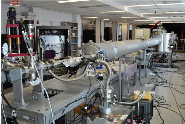
Figure 2. The MIT polarimetry beamline. On the far left of the image, the source chamber contains the high voltage Manson source, which is shining onto an LGML mounted on a translational and rotational stage. Reflected, polarized light then travels down the beamline into the grating chamber, where it is attenuated into a slit and incident on gratings mounted in the chamber. The light is dispersed by the grating and travels down the beamline to the detector chamber containing our CCD package.
