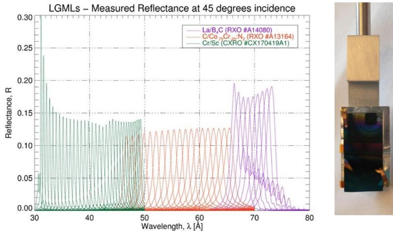
Figure 4. Left: X-ray reflectivity of three different types of multilayers measured at regular spacings across the surface of the multilayers. A mosaic of these mirrors will provide good reflectivity across the entire bandpass of the flight instrument. Right: an image of the LGML currently in use in the system. It is mounted on a translational stage to allow selection of energy for the reflected X-ray beam.
