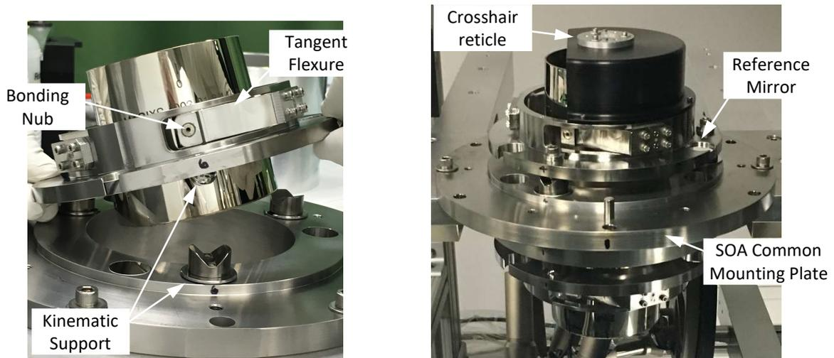
**Figure 3:** MaGIXS Spectrometer Optics Assembly (SOA)
