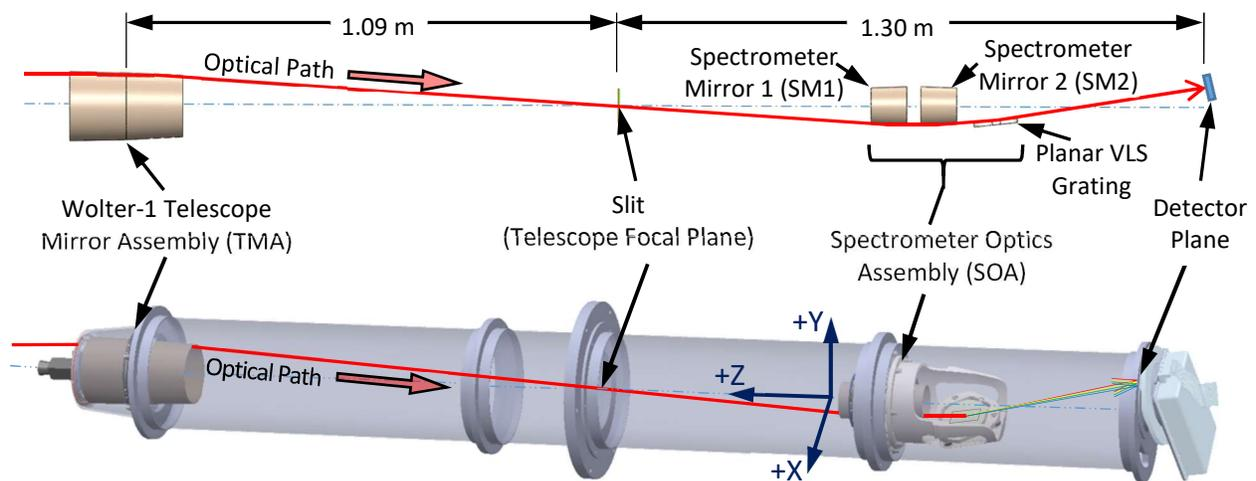
**Figure 1:** Layout of the MaGIXS Optical System
