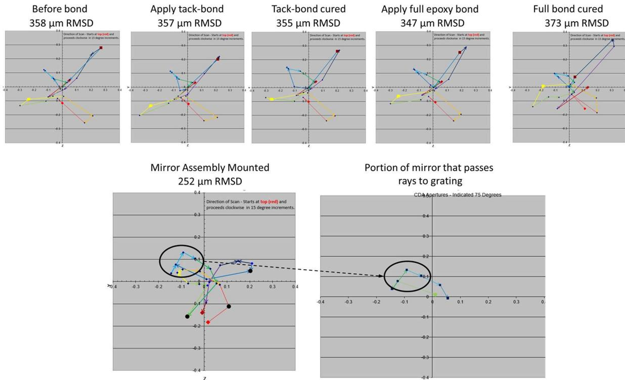
**Figure 8:** CDA Alignment Scans for Spectrometer Mirror Bonding (SM2)
