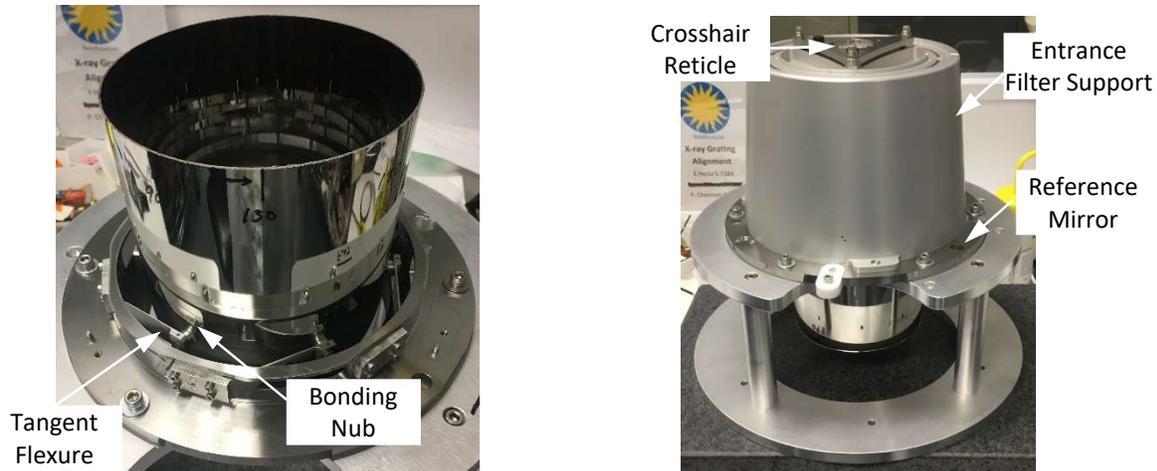
**Figure 2:** MaGIXS Telescope Mirror Assembly (TMA)
