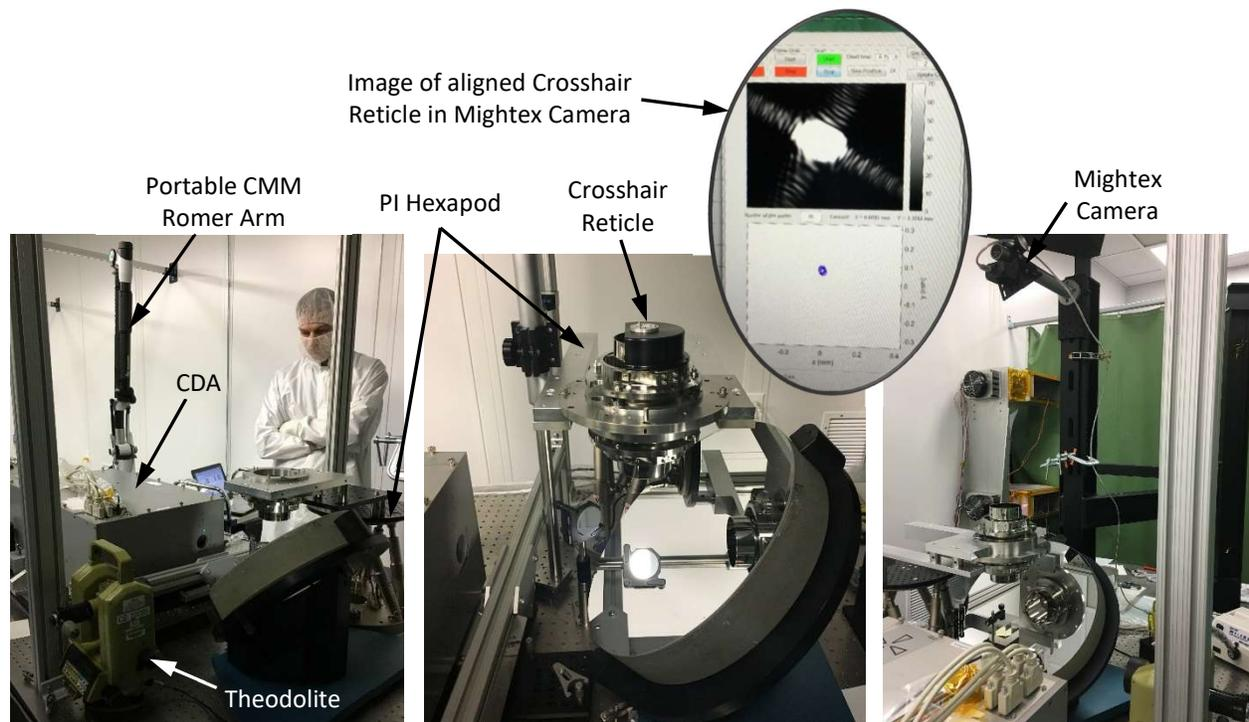
**Figure 10:** Aligning the SOA
