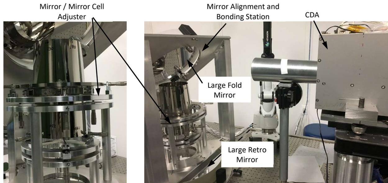
**Figure 7:** Aligning and Bonding the TMA
