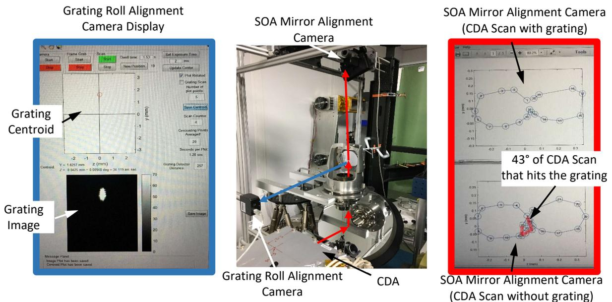
**Figure 12:** Aligning the Grating
