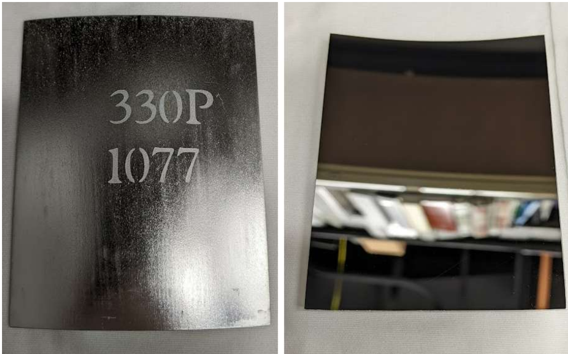
Figure 3-5 Images of Mirror Coated With 20nm Platinum Using ALD
