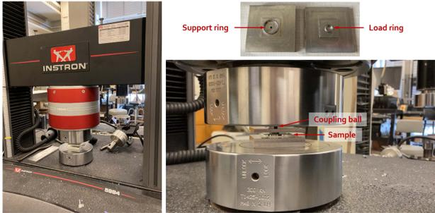
**Fig. 9.** Photographs of silicon wafer strength testing setup with an Instron machine using ring-on-ring test. Left: Instron machine used to apply the monotonic loading. Top right: support ring plate and load ring plate made of stainless steel. Bottom right: a pair of sample holders supports the specimen between two load cells in the Instron machine.
