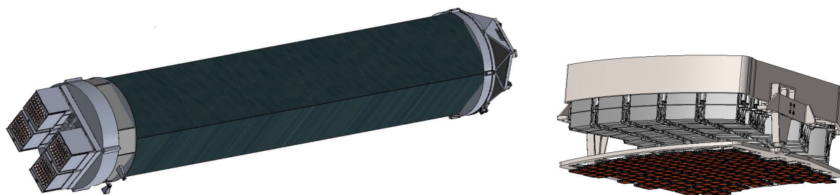
Figure 1. Left: Schematic of the Arcus XRS after deployment. X rays enter the forward assembly from the left into four parallel OCs through thermal precollimators, followed by SPO and CAT grating petals (not visible), propagate through the extendable boom, and are detected by CCD cameras mounted to the rear assembly (RA) on the right. The RA is mounted to the same deck as the UV spectrometer (not shown). Right: Perspective view of a SPO (top) and grating (bottom) petal pair. The grating petal is curved to follow a prescribed Rowland torus surface.
