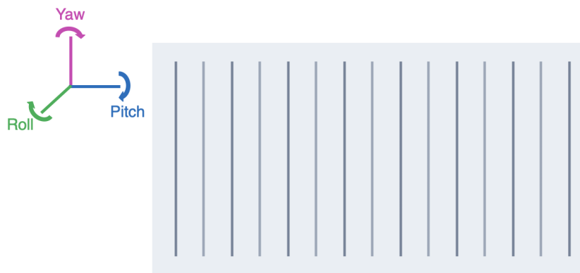
Figure 3. Definition of the local pitch, yaw, and roll angles used to describe CAT-grating orientation. The grating is represented face-on along its surface normal, with its long side along the x -axis and its short side along the y -axis. The lines parallel to the y -axis schematically represent the CAT-grating bars; their spacing and number are not shown to scale. Pitch is a rotation about the in-plane x -axis, yaw is a rotation about the orthogonal in-plane y -axis, and roll is a rotation about the surface normal pointing out of the page.
