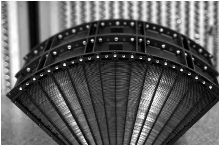
Figure 1-3: A quadrant composed of 168 nested foil mirrors. The radial bars are oriented perpendicularly to the foils, holding them in place.
