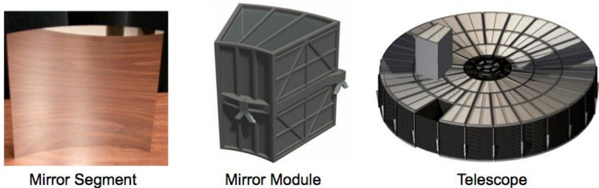
Figure 1.4 Module concept for large x-ray observatory optics assembly. Many mirror segments are assembled into a module and accurately co-aligned. The modules are then combined into a full optic assembly and again co-aligned. Images from [4].
