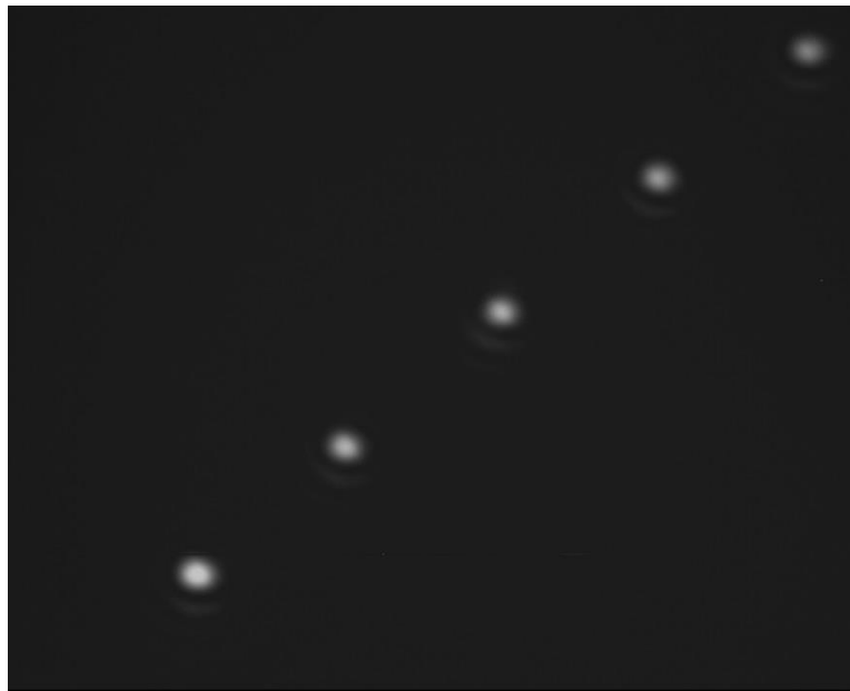
Figure 2.13 Image of focal spots on CCD. The centroids of these spots are tracked throughout the experiment.
